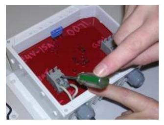
The combo rectifier/regulator has two terminal blocks: one with three terminals (for the cable from the turbine) and one with two terminals (for the cable to the battery).
