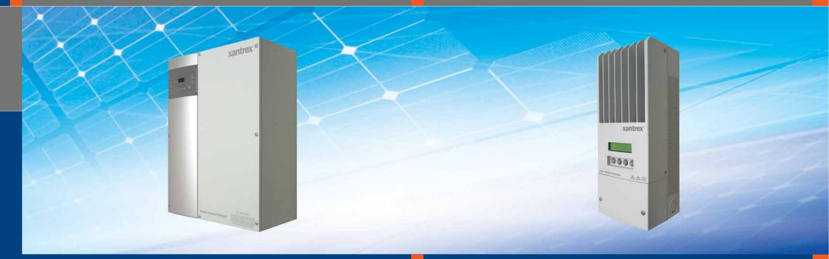
The XW Hybrid Inverter/Charger (XW) is a true sine wave inverter/charger that incorporates a DC to AC inverter, a battery charger, and an AC auto-transfer switch. It is the foundation for battery-based residential applications up to 18 kilowatts (kW), and commercial applications up to 36 kW in a three-phase configuration. Designed for off-grid and back-up applications, the XW can operate with generators and renewable energy sources to provide reliable power every time.
