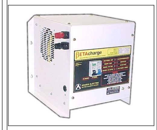
The WOODS ELECTRIC BETAcharge II is a sophisticated electronic multiple-taper charger for most types of batteries. It employs microprocessor-controlled SCRs to precisely regulate charging voltages and currents during all phases of charging. The BETAcharge II successfully charges deeply discharged batteries and batteries which are loaded during charging. The BETAcharge II will not overcharge batteries which are already fully charged.
